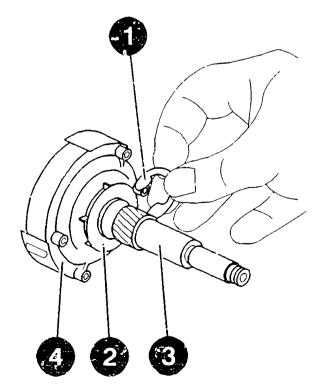
Checking planetary gear train
